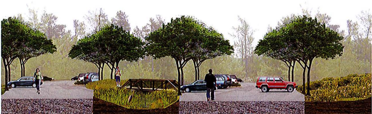
Cross-section of parking lot with bio-swales
